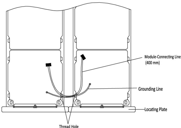
Figure 3-52 Place the Grounding Line and Module-Connecting Line
