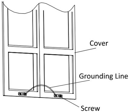
Figure 3-57 Connect the Grounding Line to the Cover
