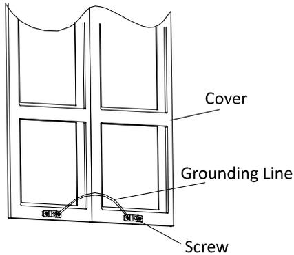
Figure 3-47 Connect the Grounding Line to the Cover
