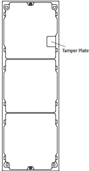
7. Fill and level up the gap between the frame and wall with concrete. Remove the locating plates after the concrete is dry.
