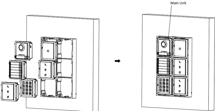
Figure 3-46 Insert the Modules
