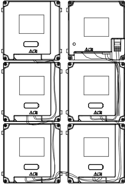
Figure 3-45 Line Connection Effect Picture
