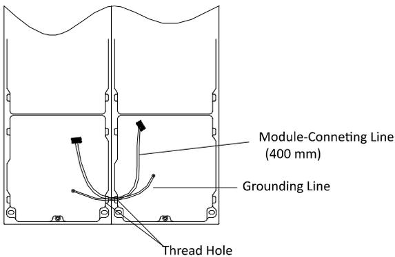
Figure 3-42 Place the Grounding Line and Module-Connecting Line
