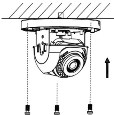
Figure 2-5 Fix the Mounting Base
