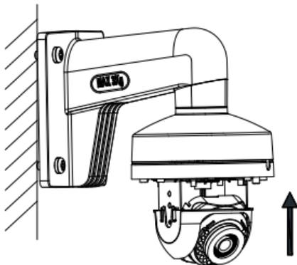
Figure 2-16 Fix the Camera to Wall Mounting Bracket
