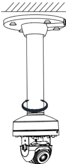
Figure 2-19 Install the Cap
