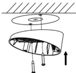
Figure 2-21 Fix Incline Mounting Bracket to Wall
