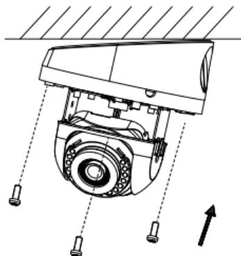
Figure 2-22 Fix the Camera to Incline Mounting Bracket
