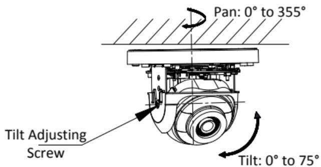
Figure 2-9 Type IV Camera 2-Axis Adjustment
