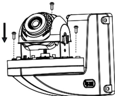
Figure 2-12 Fix the Camera to Wall Mounting Bracket
