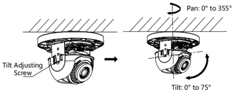
Figure 2-6 Type I Camera 2-Axis Adjustment
