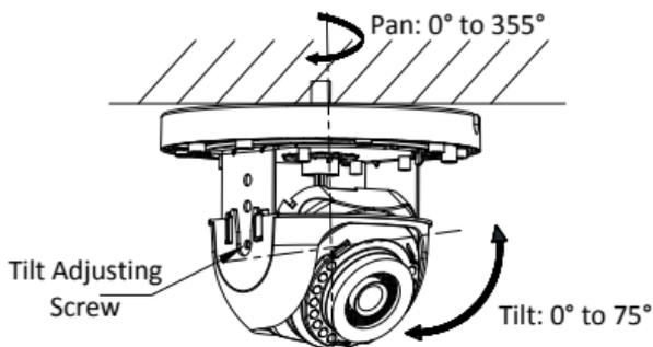
Figure 2-8 Type III Camera 2-Axis Adjustment
