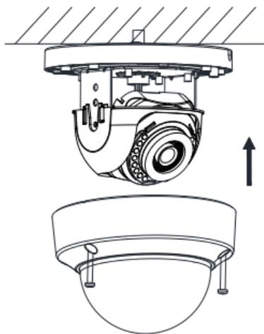
Figure 2-10 Install Bubble
