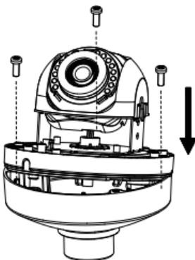
Figure 2-18 Fix the Camera to Cap
