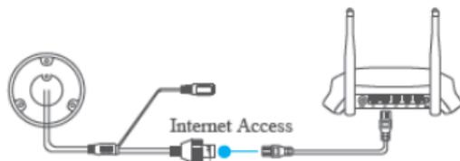
Figure 5-3 Connect a Router
