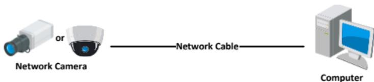
Figure 3-1 Connecting Directly
