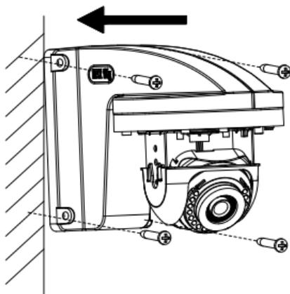
Figure 2-13 Fix the Wall Mounting Bracket to Wall
