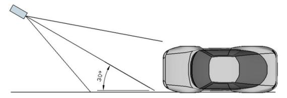
Install the camera to the front of the vehicle (Recommended). If you want to recognize two lanes - it is generally recommended to mount a camera on a crossbar.
