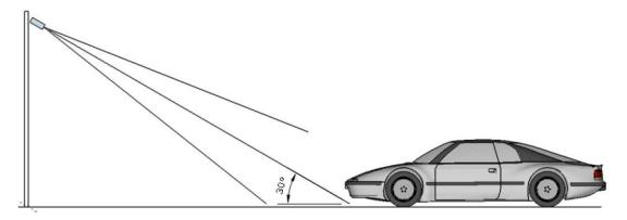
The view angle of the camera should be within 30 degrees to the path of movement. Horizontal angle - should not exceed 30 degrees
