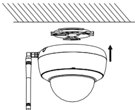
Figure 2-3 Secure the Camera to the Adapter Plate
