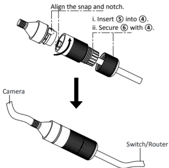
Figure 2-9 Water-proof Accessory Installation
