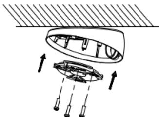
Figure 2-6 Secure the Adapter
