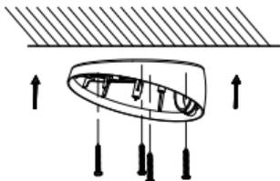
Figure 2-5 Secure the Bracket
