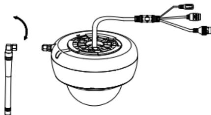
Figure 2-1 Mount the Wi-Fi Antenna
