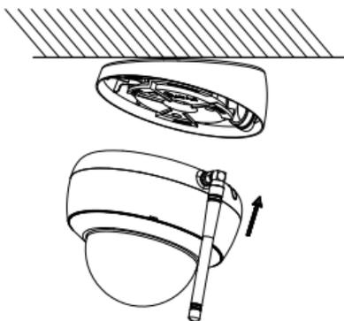
Figure 2-7 Secure the Camera to the Adapter Plate
