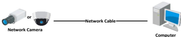
Figure 3-1 Connecting Directly
