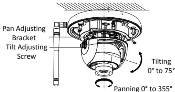
Figure 2-4 Adjust the View Angle
