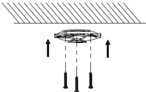
Figure 2-2 Install the Adapter Plate to the Ceiling
