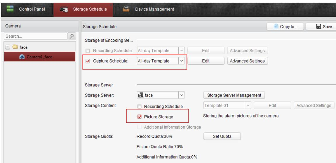
Step 4: Enter [Device Management]-[Remote Configuration]. Face detection function can be configured in VCA Config. The configuration is same with the way in the web.
