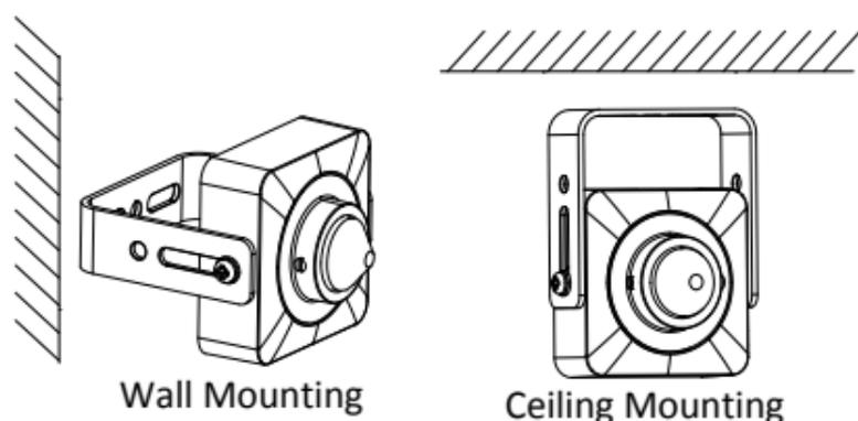
Figure 2-1 Wall Mounting and Ceiling Mounting
