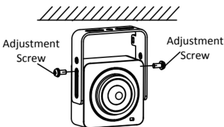
Figure 2-4 Loosen the Adjustment Screw
