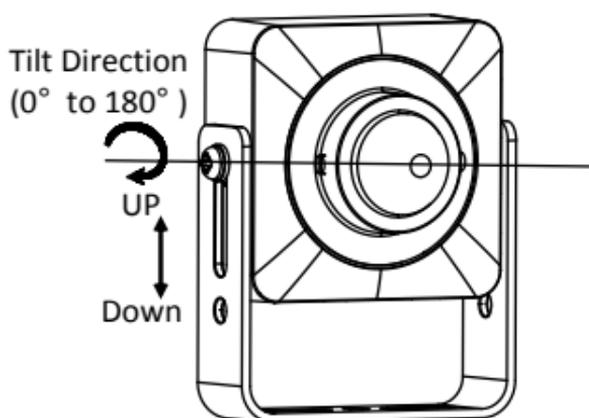
Figure 2-5 Adjust the Angle
