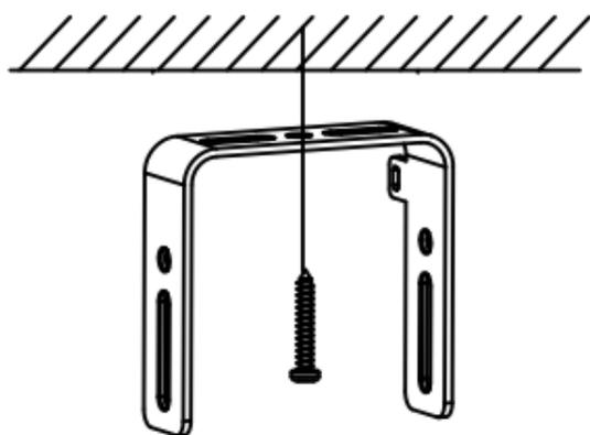
Figure 2-3 Install the Bracket
