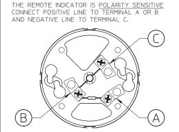
DETECTOR RANGE CONNECTIONS SERIES 60 INTRINSICALLY SAFE XP95 INTRINSICALLY SAFE DISCOVERY ALARMSENSE ORBIS VOLTAGE, A & C 5 - 36V 25mA, UP TO 40°C MAX CURRENT, B & C OPERATING TEMPERATURE -10° TO +60°C
