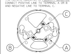
DETECTOR RANGE CONNECTIONS SERIES 60 INTRINSICALLY SAFE XP95 INTRINSICALLY SAFE DISCOVERY ALARMSENSE ORBIS VOLTAGE, A & C MAX CURRENT, B & C 25mA, UP TO 40°C OPERATING TEMPERATURE -10° TO +60°C
