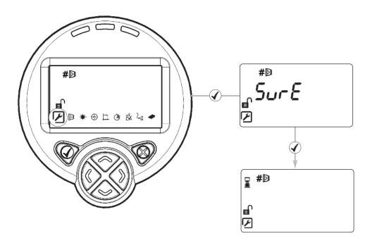
If it is not known where the beam is pointing, use Home Position to automatically steer the infrared beam to approximately the centre of its range of movement.
