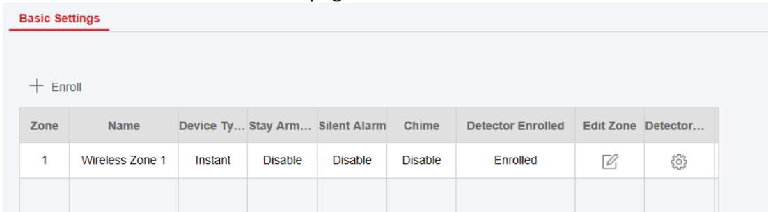
The screenshot shows the 'Basic Settings' page with a '+ Enroll' button and a table of zones. The table has columns for Zone, Name, Device Ty..., Stay Arm..., Silent Alarm, Chime, Detector Enrolled, Edit Zone, and Detector... The first row shows Zone 1, Name 'Wireless Zone 1', Device Type 'Instant', Stay Arm 'Disable', Silent Alarm 'Disable', Chime 'Disable', and Detector Enrolled 'Enrolled'. There are edit and settings icons in the last two columns.
