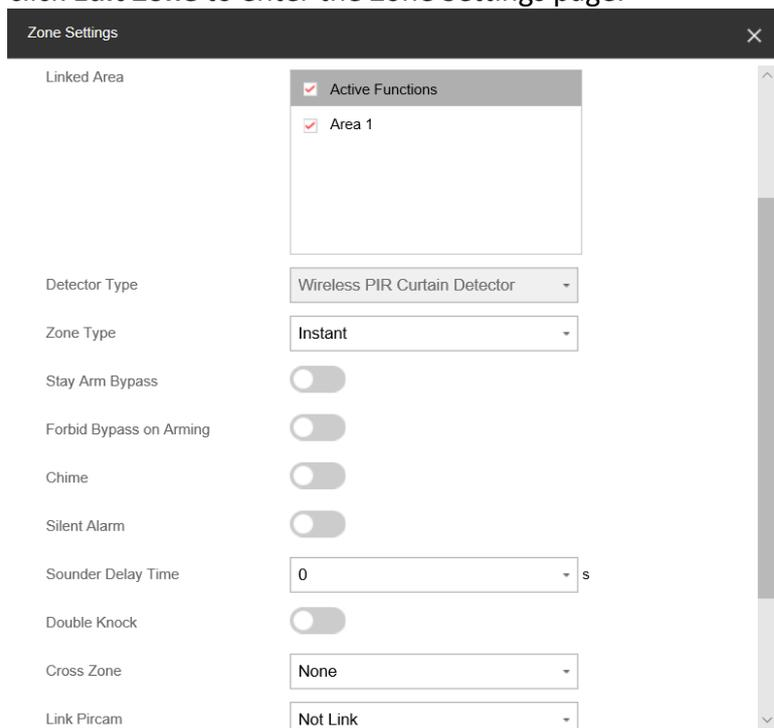
The screenshot shows the 'Zone Settings' page. It has a 'Linked Area' section with a list of areas (Area 1) and a 'Detector Type' dropdown set to 'Wireless PIR Curtain Detector'. Other settings include 'Zone Type' (Instant), 'Stay Arm Bypass' (off), 'Forbid Bypass on Arming' (off), 'Chime' (off), 'Silent Alarm' (off), 'Sounder Delay Time' (0 s), 'Double Knock' (off), 'Cross Zone' (None), and 'Link Pircam' (Not Link).
