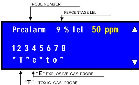
Press the **"DX"** and **"SX"** buttons and move to the desired probe, (in the drawing the 4).
