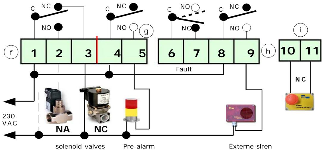
==== Normally Closed Solenoid Connections with Positive Safety =====
