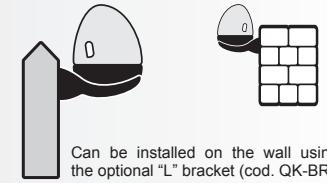
Can be installed on the wall using the optional "L" bracket (cod. QK-BRALUX)
